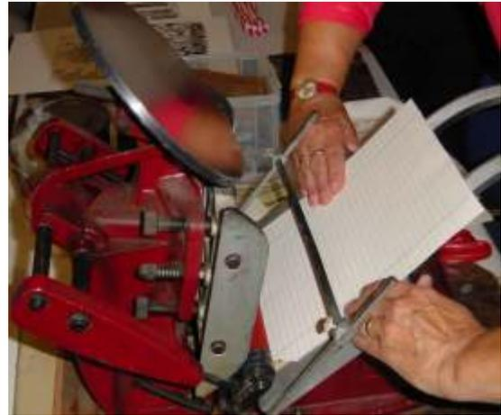
At this stage the chase was not yet in the press. A few blobs of ink was smeared onto a few places on the ink disk. Then, by pushing the handle down and up, the rollers moved over the disk, the disk itself rotates, spreading the ink as it goes. If you rotate the disk manually in addition to the machine rotated the disk, you speed up the process, and very soon there was a nice, thin, even layer of ink on the disk.
